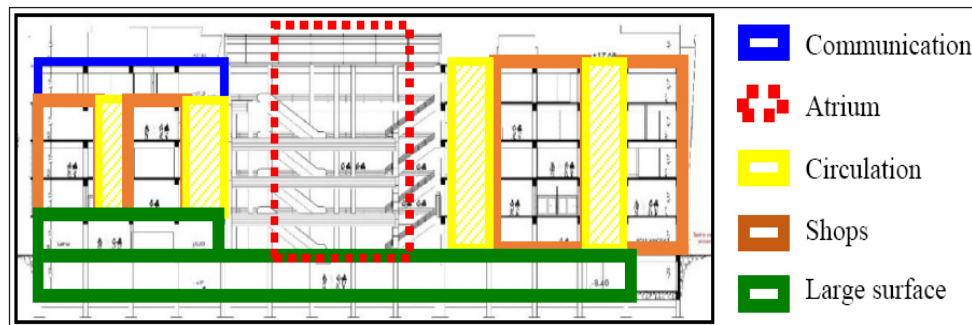
Figure 6. Typical section of the different levels illustrating the services of the Ritej mall (Source: Office of architecture Hammou Dziri Hammou, 2020 ).
